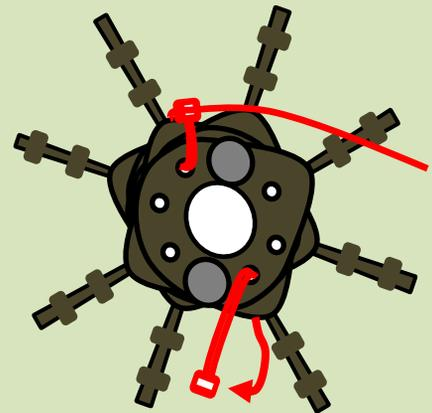
Secure the Stars together by inserting two Cable Ties through the Small Holes that are opposite each other on the Legs. Wrap the Cable Tie loop to the outer edge and not through the large center hole. Connect and trim the ends of the Cable Ties as needed. (Note: The correct way to connect the Cable Tie-See Below)
