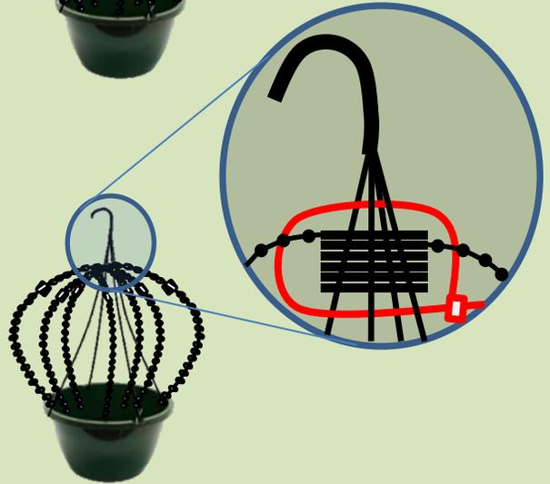
Lace Cable Tie through the wire hanger strands above the trellis and connect under the trellis assembly. Trim the ends of the Cable Tie as needed. This will finish the Project!
